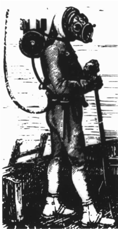
Figure 1.3 The aerophore, devised by Rouquayrol and Denayrouze, 1865. This device was widely used and was an important milestone in the development of the modern scuba.
